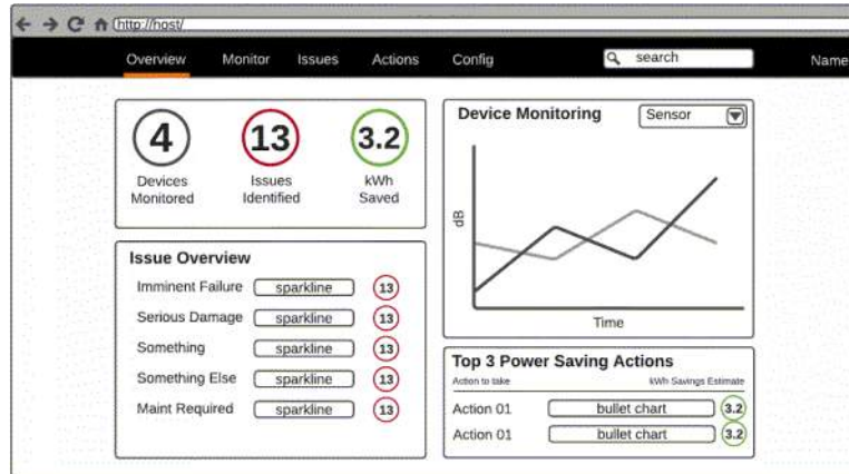
Figure 4: Mock-up of the user interface for the portal web page, allowing users to view problems with machinery, look at aggregated data, and record fixed issues.
